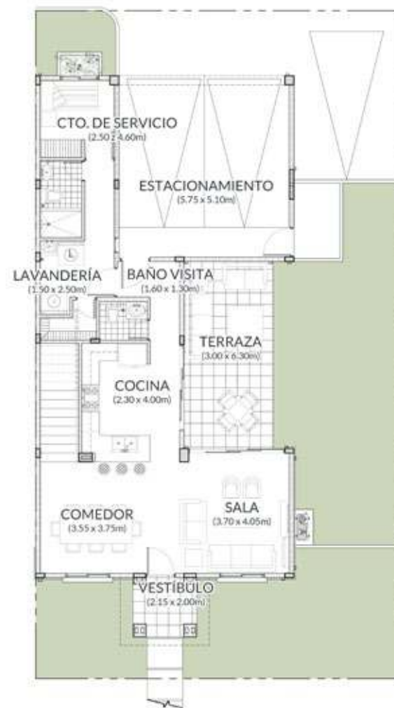
Planta baja / Ground Floor
